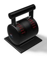
The BUK-H has been designed with a zero build-in depth, for the desktop mounted shape with potentiometers. It is also suitable for transverse thruster control due to its symmetrical and therefore applicable in various orientations. The basic signal transmitters are dual 5KOhm potentiometers that return 10-90% of the supply voltage over the full lever travel of 120°.
