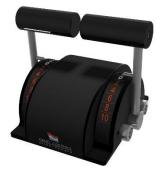
The BUK-G mk2 is the **IP68 level** model of the BUK-G and has been especially designed for applications in yachting. It has a slightly different shape compared to the standard BUK-G, to be protected from immersion in water with a depth over 1 meter. The BUK-G mk2 is suitable for both propulsion and transverse thruster control. The basic signal transmitter is a 2KOhm potentiometer that returns 10-90% of its supply voltage over the full lever travel of 120°.
