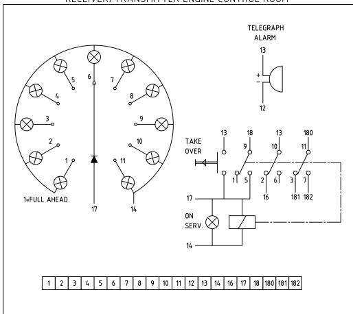
WIRING DIAGRAM RECEIVER/TRANSMITTER E.C.R.
