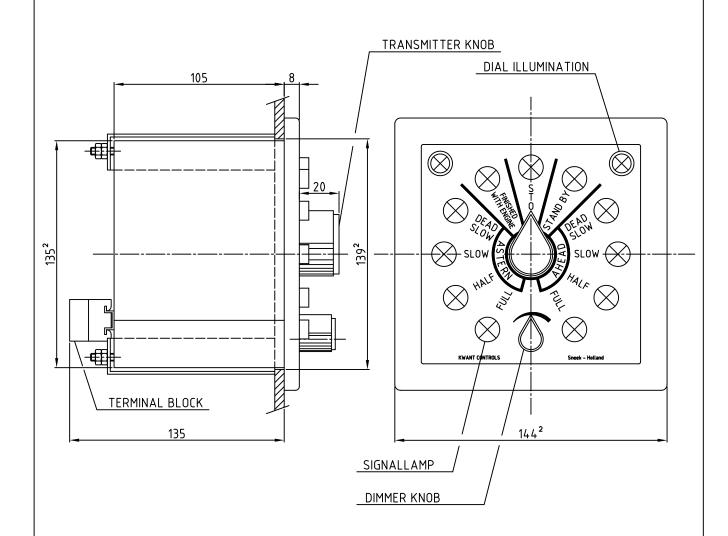
TRANSMITTER RECEIVER WITH LAMP SIGNALLING
