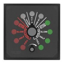
The "Norm" type telegraph has been designed to be used on board of all types of vessels having a remotely controlled propulsion control, and serve as the back-up communication system in case the remote control system should fail. The wheelhouse and engine control room telegraphs are console mounted, IP42, 144x144mm devices, and have a stainless steel housing and a non-reflective black finish. An IP56 housing is available for bulkhead mounting applications such as the Engine Room.
