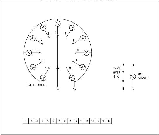
WIRING DIAGRAM RECEIVER/TRANSMITTER ENGINE ROOM
